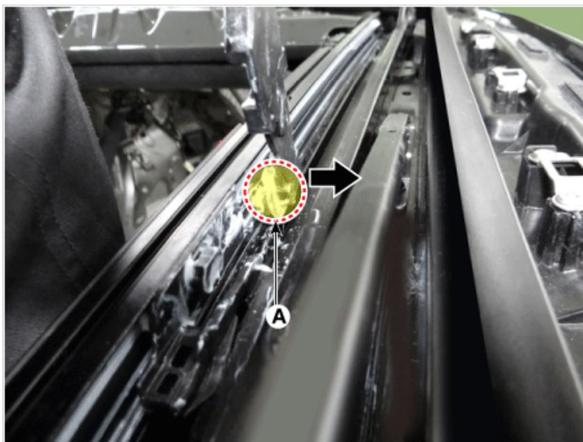
8. Remove the mechanism assembly(A) by pulling direction of an arrow.
