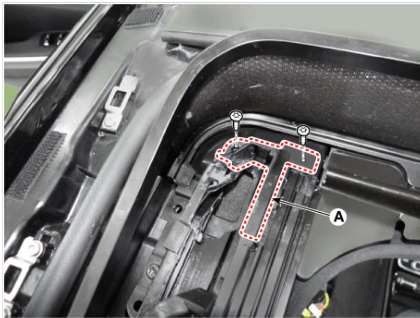
4. Move the mechanism bracket(A) to (B) spot by operating sunroof switch.
