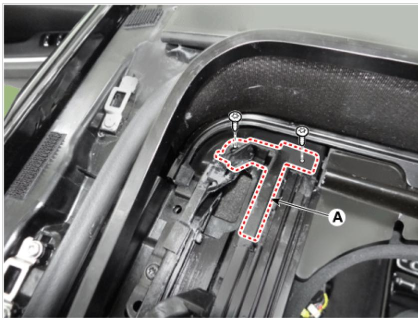
4. Move the mechanism bracket(A) to (B) spot by operating sunroof switch.
