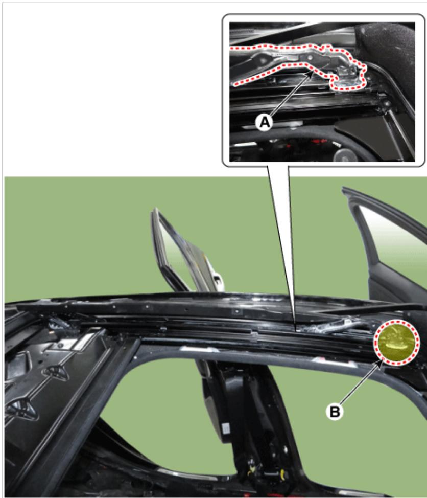
5. Remove the mechanism shoe(A) from mechanism guide by pulling direction of an arrow.
