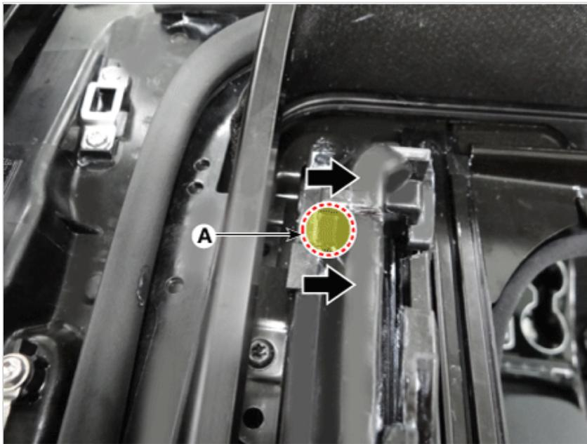
6. Place the front slide shoe(B) as picture below by pushing the mechanism assembly(A) direction of an arrow.
